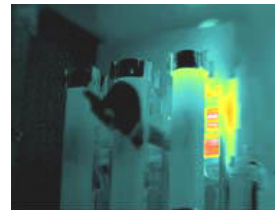
Fuse Switch Component Failure
