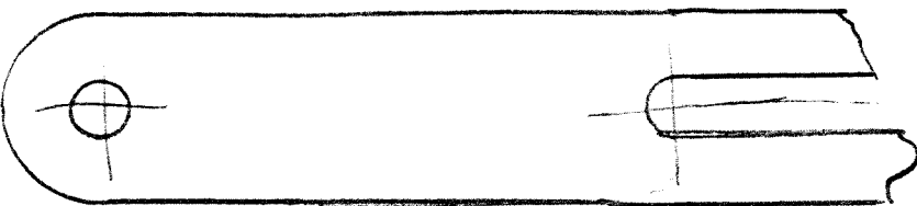
BELT TENSION REGULATING BRACKET (AS PER MOTOROLA ALTERNATORS.)
